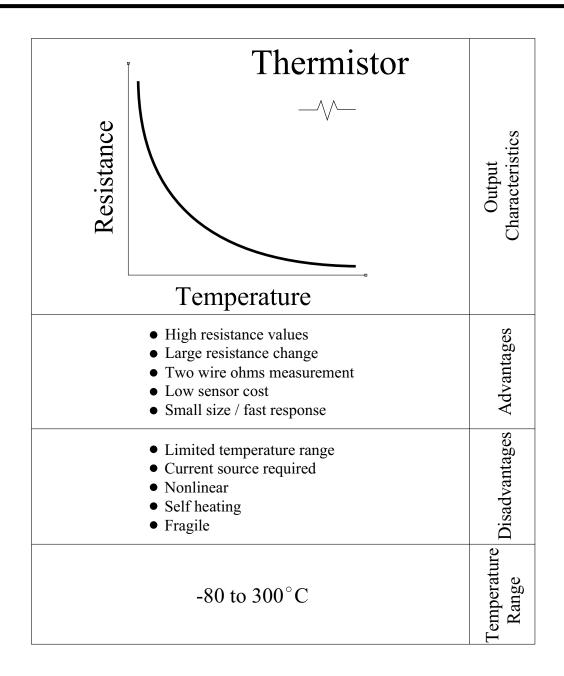
Thermistors are constructed with metal oxides formed into a bead and encapsulated in epoxy or glass. The resistance of a Thermistor has a nonlinear large negative change as it is heated (Negative temperature coefficient). The change in resistance during a temperature change of a Thermistor is several times greater than an RTD making measurement easier, but the temperature range is limited.
