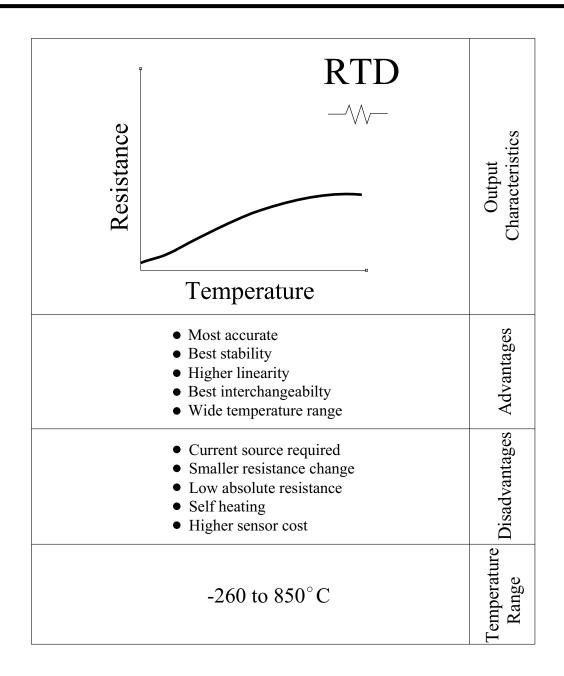
Resistance Temperature Detector's (RTD's) are constructed with a wire coil or a thin layer of metal to form a precision resistor. The resistance value changes very accurately and repeatedly in a positive direction when heated (Positive temperature coefficient). RTD assemblies can be used in a wide variety of configurations for all industries to give the highest accuracy of temperature measurement.
