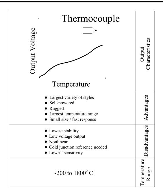
Thermocouples are constructed of two dissimilar metals welded together to form a junction. When this junction is heated there is a thermoelectric potential (emf) created on the millivolt level. The heated junction when compared to a reference junction (same junction type at a known temperature, usually  $0^{\circ}$ C) has an output proportional to the difference in the two junctions temperatures.
